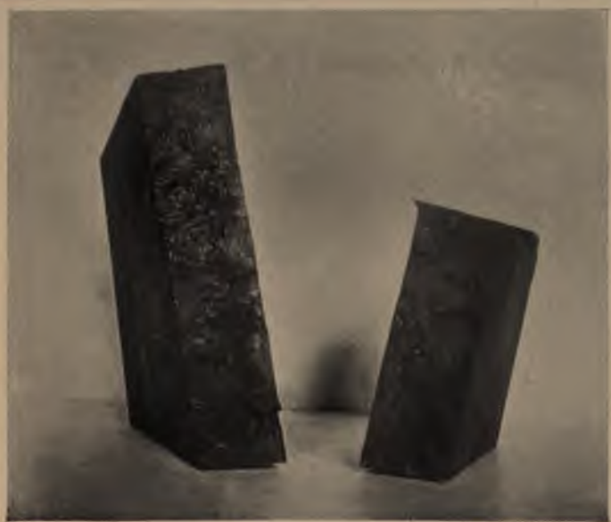
BURNED METAL OF SCHOEN STEEL WHEEL
